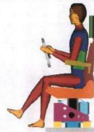
Vibration analysis of an occupied car seat
